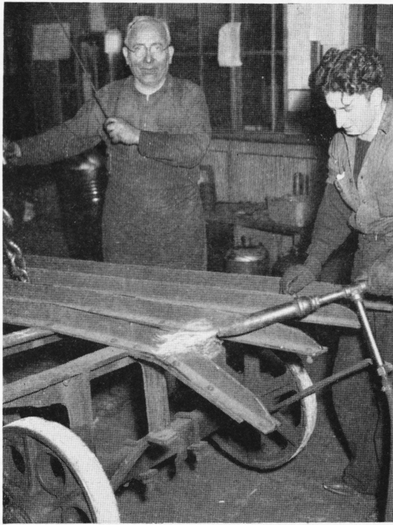
The wear and tear on muffle pans in the Mills is something tough even on tough steel. The heat of the fire, heavy bars of metal and the tug of the winch often breaks parts of the muffle pans. Instead of the Scrap Drive, they go to the Blacksmith Shop. Mike Fitzmaurice and Phil Gaudiosi do the honors.
