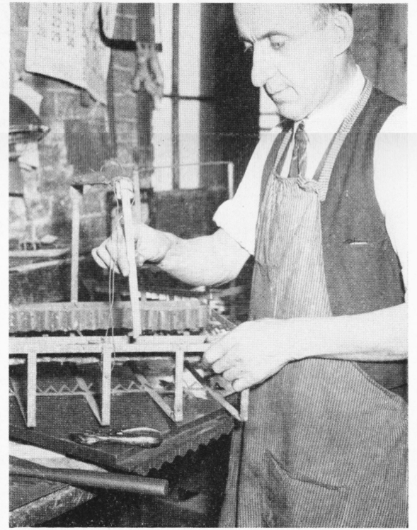
The acids and other chemicals in the Dip Room raise Cain with the metal dipping baskets. But a quick trip to the Repair Department puts them back into shape for use in production. Leo Pelletier fits a new piece to one of the baskets at his bench. Few are the ailments the Repair Room boys can't fix.
